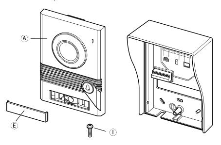
10. Choose a suitable location to attach the rain cover to a wall using the included screws.
