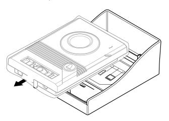
9. Remove the nameplate and bottom screw from the Outdoor video doorbell.
