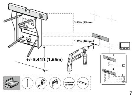
11. Attach the rain cover to the wall and prepare the wires for connection with the indoor monitor.
