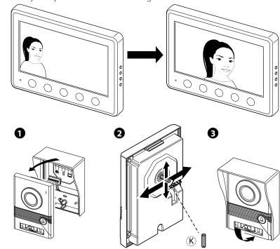
14. Once finished, insert the angle adjuster into the bottom of the rain cover and attached the camera back onto the rain cover.
