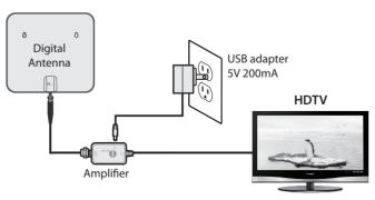
\*USB Power Cable may also be plugged into any available USB port on HDTV as well.
