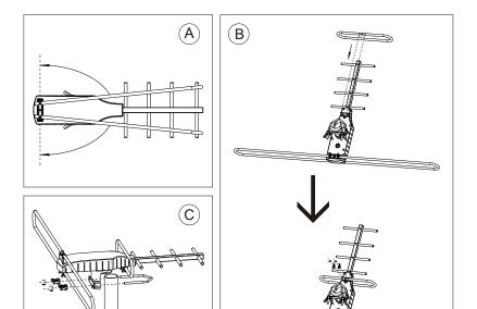
**Step 1**: Unfold the antenna booms until they stay in horizontal orientation. (Refer to graph A and B)
