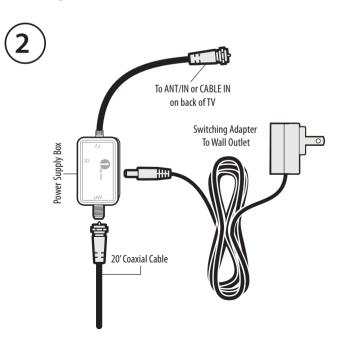
**C.** Connect the coaxial cable from the power supply box to the **ANT/IN** or **CABLE IN** port on the back of your TV (as shown in figure **3**). Note: For TV's that require a tuner box, connect the coaxial cable from the power supply box to the tuner box ANT/IN or CABLE IN port.
