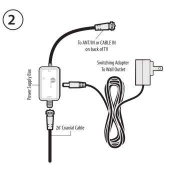
**C.** Connect the coaxial cable from the power supply box to the **ANT/IN** or **CABLE IN** port on the back of your TV (as shown in figure **3**). Note: For TV's that require a tuner box, connect the coaxial cable from the power supply box to the tuner box ANT/IN or CABLE IN port.
