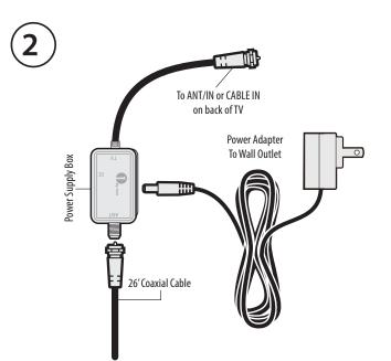
**C.** Connect the coaxial cable from the power supply box to the **ANT/IN** or **CABLE IN** port on the back of your TV (as shown in figure **3**). Note: For TV's that require a tuner box, connect the coaxial cable from the power supply box to the tuner box ANT/IN or CABLE IN port.
