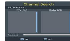
If no channel can be found during the channel search process, check the antenna connections and make sure the antenna is in proper working order. After the scanning process is complete, the converter box will automatically save the scanned channels and display the first channel from the list.
