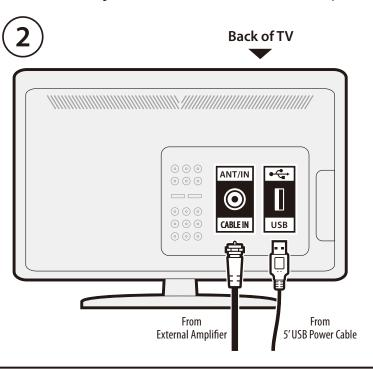
**C.** The amplifier requires power to operate properly. Plug the round end of the amplifier's 5ft. long USB power cable into the amplifier (as shown in figure **1**). Then insert the USB plug into an open USB port on the back of your TV (see figure **2**). If no USB port is available, use the supplied power adapter to power the amplifier through any standard 110V outlet (see this option in figure **3**).
