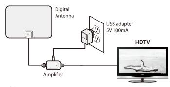
$<sup>^*</sup>$ USB Power Cable may also be plugged into any available USB port on HDTV as well.
