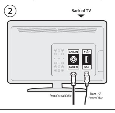
**C.** The amplifier requires power to operate properly. Plug the round end of the amplifier's USB power cable into the amplifier (as shown in figure **1**). Then insert the USB plug into an open USB port on the back of your TV (see figure **2**). If no USB port is available, use the supplied power adapter to power the amplifier through any standard 110V outlet (see this option in figure **3**).
