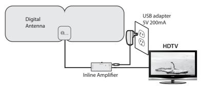
$^{*}$ USB Power Cable may also be plugged into any available USB port on HDTV as well.
