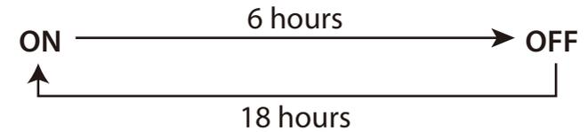
● **1-6H setting:** The user can also set the timer as 1H, 2H, 3H, 4H, 5H, or 6H using the remote control.
