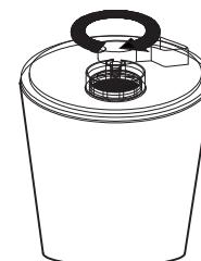
3. Remove the cap and the attached filter.
