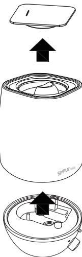
1. Remove the vapor nozzle from the water tank.
