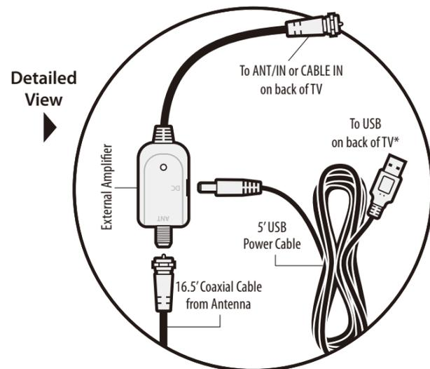
**B.** Connect the coaxial cable from the amplifier to the **ANT/IN** or **CABLE IN** port on the back of your TV (as shown in figure 2). Note: For TV's that require a tuner box, connect the coaxial cable from the amplifier to the tuner box ANT/IN or CABLE IN port. See the "Final Configuration" illustrations below for both connection options-
