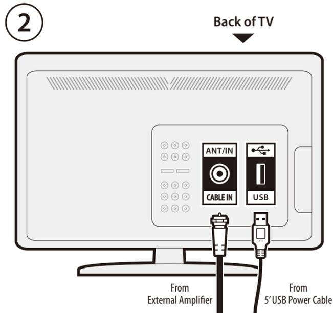
**C.** The amplifier requires power to operate properly. Plug the round end of the amplifier's 5ft. long USB power cable into the amplifier (as shown in figure 1). Then insert the USB plug into an open USB port on the back of your TV (see figure 2). If no USB port is available, use the supplied power adapter to power the amplifier through any standard 110V outlet (see this option in figure 3).
