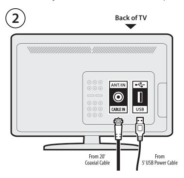
**C.** The amplifier requires power to operate properly. Plug the round end of the amplifier's USB power cable into the amplifier (as shown in figure 1). Then insert the USB plug into an open USB port on the back of your TV (see figure 2). If no USB port is available, use the supplied power adapter to power the amplifier through any standard 110V outlet (see this option in figure 3).
